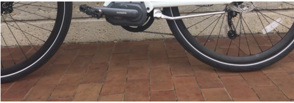
A Cannondale 2017 Kinneto with a mid-drive pedal assist motor. (Andrew Small/CityLab)
