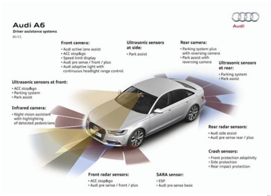
A breakdown of the 2012 Audi A6 Driver Assistance Systems shows how they help with driver awareness.
