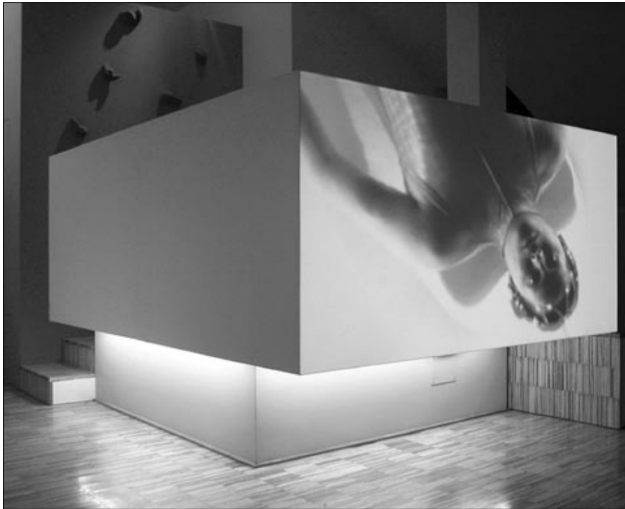
IBM's Everywhere Display is part of the 'Digital_minimal' exhibit now on display in the School of Architecture and Planning's Wolk Gallery through March 29. The installation is a video projector with a rotating mirror that allows any surface around it to become a potential screen.
